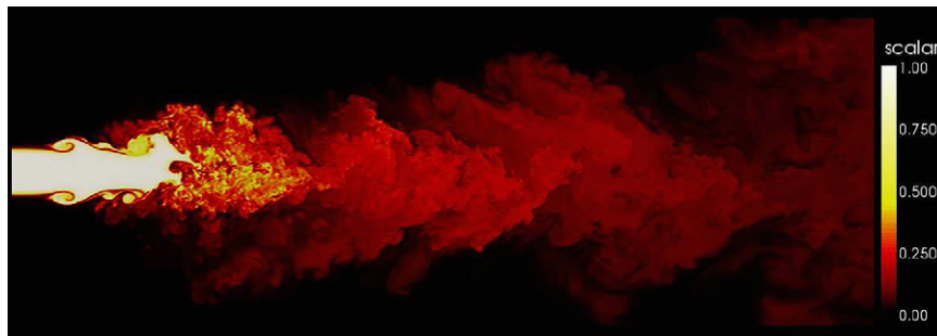
Fig. 6. Contours of a passively convected scalar for the present DNS at density ratio 1:7. The strong decay of the scalar value indicates the intense mixing processes induced by the rapid breakdown of the potential core.
