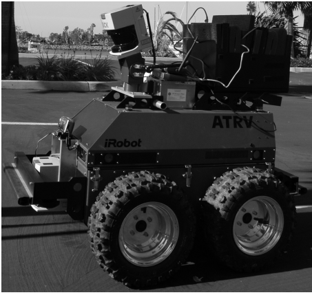
Figure 5: The ATRV robotic platform.
