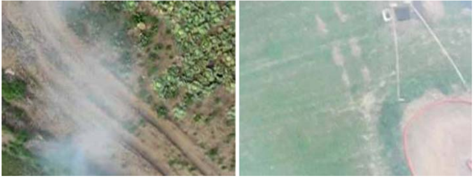
Fig. 4 Typical occlusions caused by engine smoke; camera is mounted on the bottom of the UAV and it points the terrain
