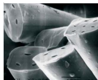
Hollow synthetic fibres viewed under a scanning electron microscope (SEM). © IFTH
