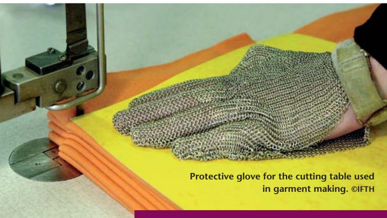
Protective glove for the cutting table used in garment making. ©IFTH
