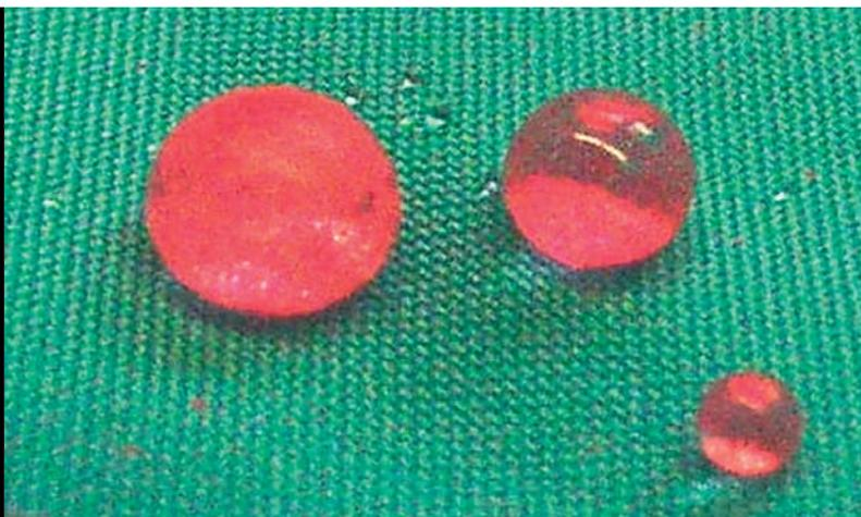
The self-cleaning and hydrophobic properties of textiles manufactured using the nanotechnological process known as the Lotus effect®. ©V.v.Arnim-ITV Denkendorf
