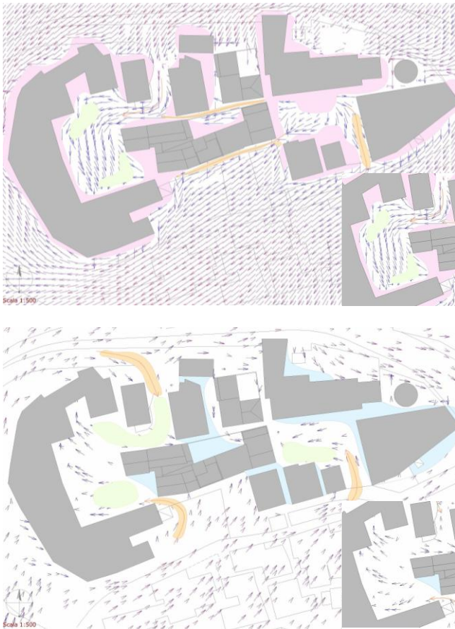
Fig. 4 The summer ventilation (above); the winter ventilation (below). In evidence, one of the part of interest for the project.
