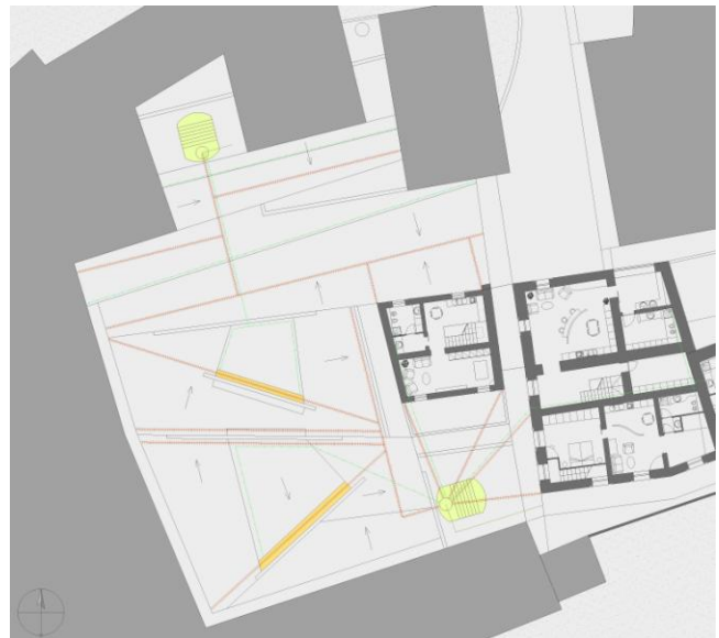
Fig. 7 Rainwater harvesting and channelization project. The system has been located below the floor level of Largo Palace. The orange lines identify the collection pipes while the green lines identify the water distribution pipes. The location of the two storage tanks is highlighted in yellow.
