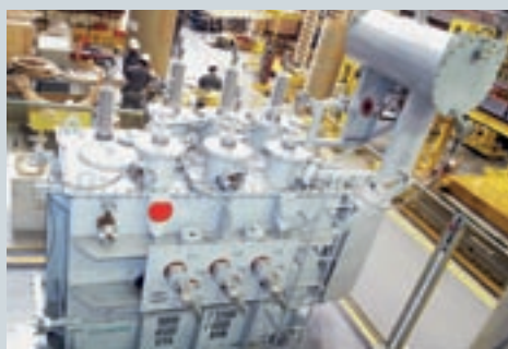
Double-tier transformer, with forced-air ventilation, 9/12 MVA, for Costa Rica
