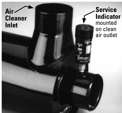
Filter service indicators are very effective when mounted on the outlet tube of the air cleaner, see The Informer™ above. This gives the operator constant and accurate visibility of filter life.
