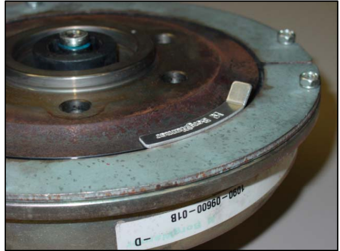
Liner Replacement Necessary
