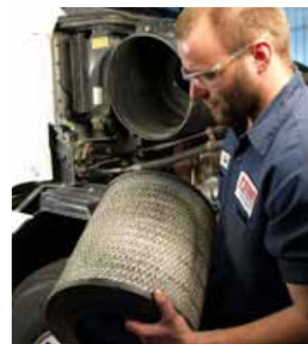
The clean side of your air filter can vary depending on the application. Some filters load on the outer surface (shown below - referred to as standard flow), and some load on the inside surfaces of the filter (referred to as reverse flow).
