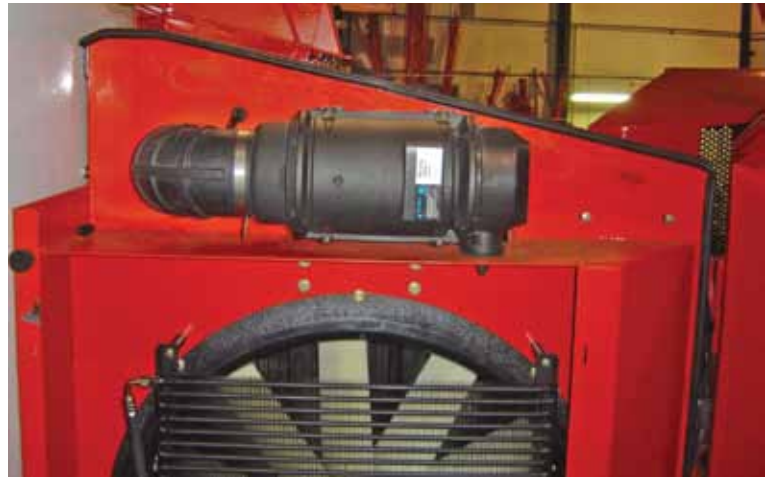
A PSD10 mounted horizontally was the equipment manufacturer's choice on this diesel-powered (285 HP @ 2,000 RPM) feller buncher.
