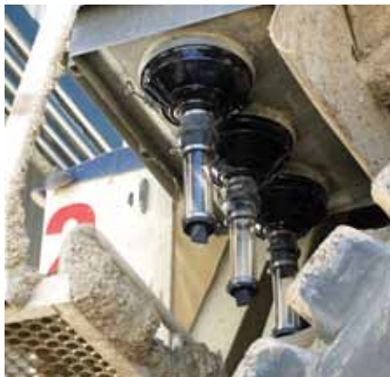
Dust Dumpa tube extensions ship fully assembled. Left: Part No. X006561 and Part No. X006562 on right.
