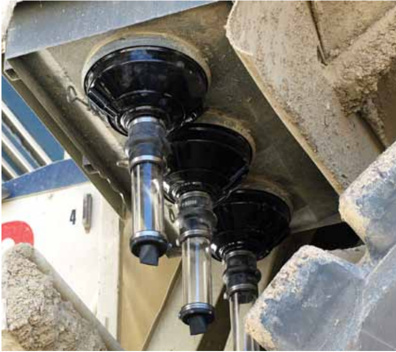
Three kits required for S Series double-inlet models. For proper performance all dust cups must have the new Dust Dumpa installed.
