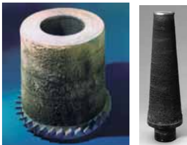
Both of these filter looks ready for replacement, but neither have reached their final servicing point.
