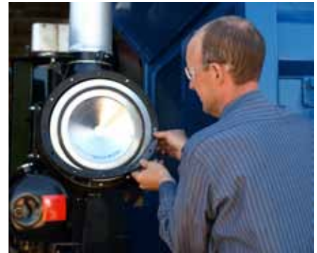
When servicing the EBB, make sure to replace the cover gasket when changing filters.
