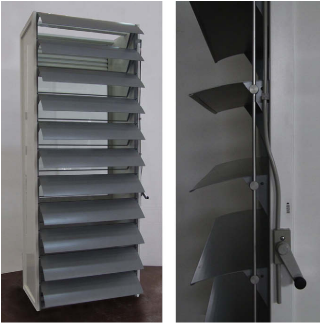
Fig. 2. Prototype of the double skin façade proposed in an open configuration.
