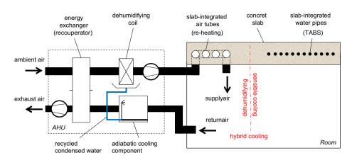
**Figure 6** Scheme of the air handling unit (AHU) and principle of hybrid cooling. Conditioning of the room with two separate systems for cooling (water based system) and for dehumidification (air-based system).
