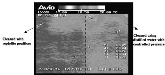
Fig. 4. Thermal image of Kapandriti's stone surface.
