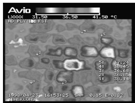
Fig. 11. Thermal image of masonry in the National Stadium of Heraklion.
